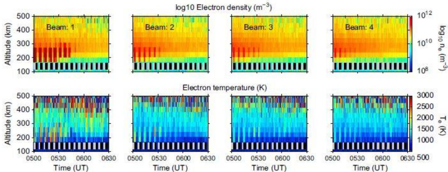
**Fig. 4.** Poker Flat Incoherent Scatter Radar observations of electron density (upper panels) and electron temperature (lower panels) with altitude in 4 different look directions from long-pulse data, post-integrated to 30.72s. HIPAS was operated in pulsed (grey panels) and continuous wave (black panels) modes with other periods having no transmissions.
