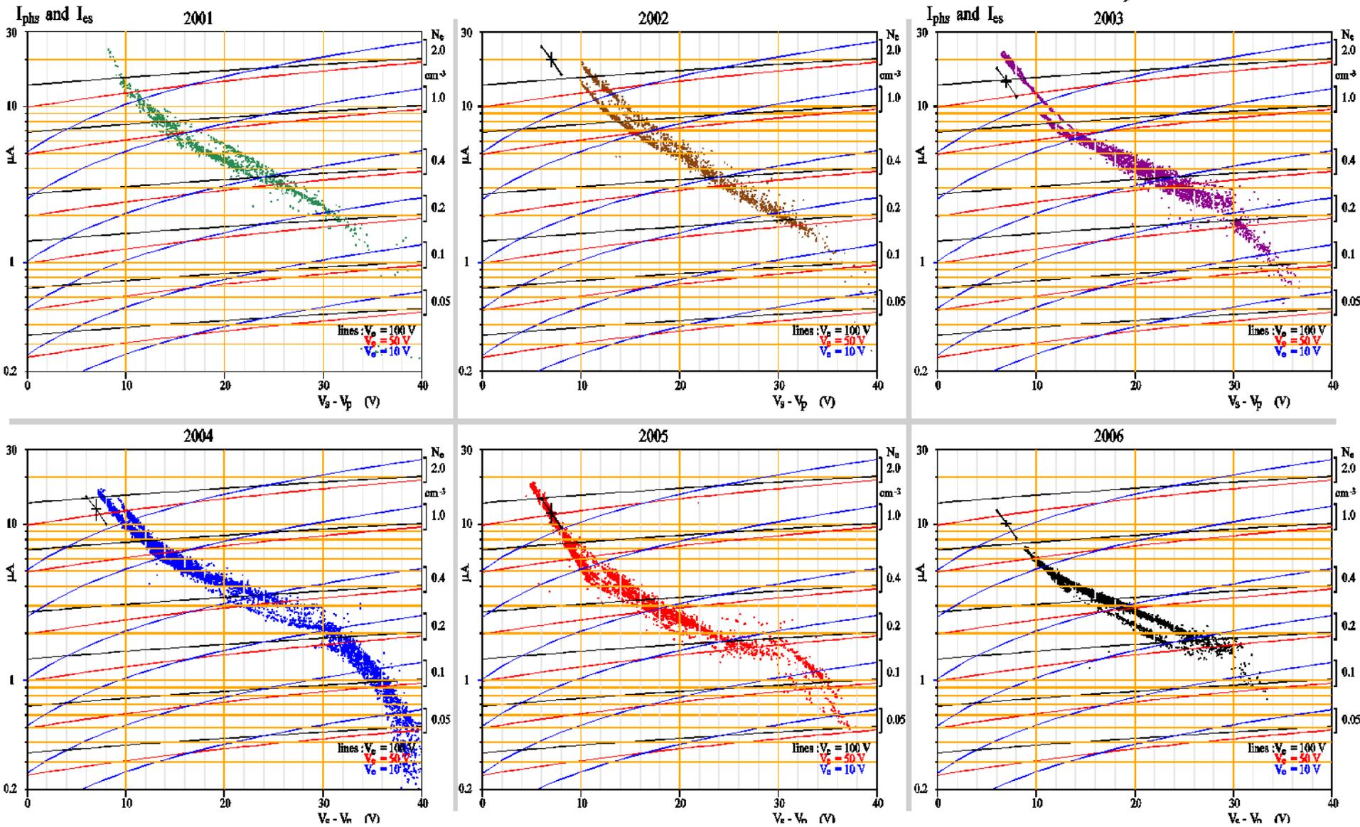
$I_{phs}$  as a function of  $V_S - V_P$  from calibrations with PEACE in the plasmashet and plasmashet boundary layer. The blue, red and black lines are calculated values of  $I_{es}$  versus  $V_S - V_P$ , for selected values of  $N_e$  and  $V_e$ . Electron densities as a function of  $V_S - V_P$  can be estimated from the crossings of scatter plots and coloured lines.
