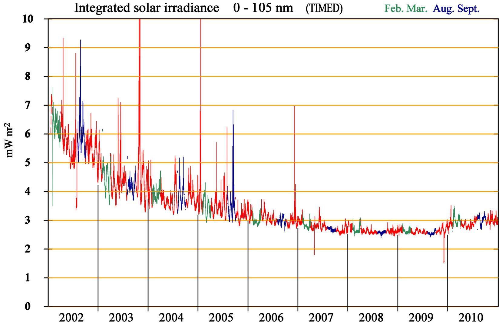
The solar EUV radiation (0–105) nm during the solar cycle from 2002 to 2010 has variations with the solar rotation period. They are more pronounced during solar maximum. A marked drop in the average radiation level has been observed, from near solar maximum to near solar minimum. **Green** parts are for early in the year (solar wind calibrations), and **blue** parts are for early autumn (plasmashet calibrations).
