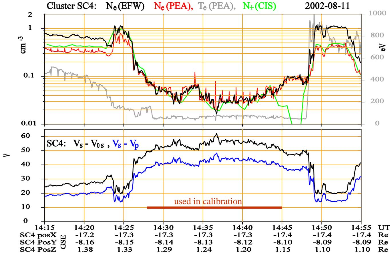
A passage of C4 from the plasmasheet to the boundary layer, and further to the lobe, provides a good opportunity to obtain a calibration of  $N_e$ (EFW). PEACE measurements of  $N_e$  are based on a complete electron energy spectrum, and the mean electron energy (grey curve in upper panel) is just below 50 eV.
