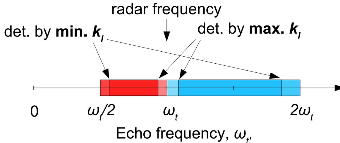
**minimal  $|\Delta\omega|$**  is determined by **max.  $k_i$**  of turbulence spectrum
