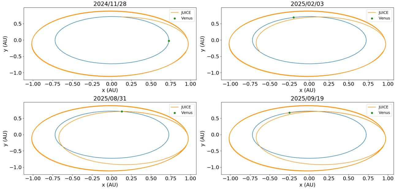
Figure 3.7: Crossing points of JUICE with the orbit of Venus and their respective dates. After launch, the spacecraft crosses through the orbit of Venus 4 times (as seen from the ecliptic plane). The Venus flyby, serving as a gravitational assist manoeuvre, can be seen in the bottom left panel.
