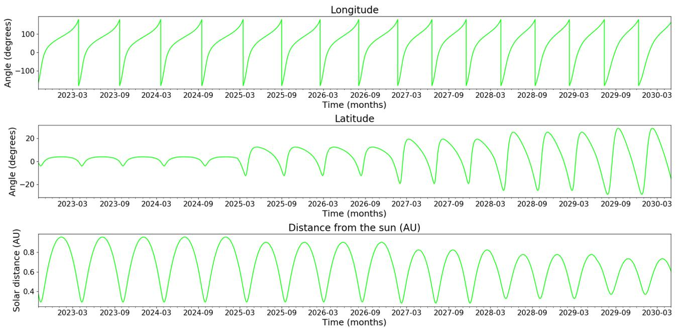
Figure 5.3: Coordinates of Solar Orbiter.
