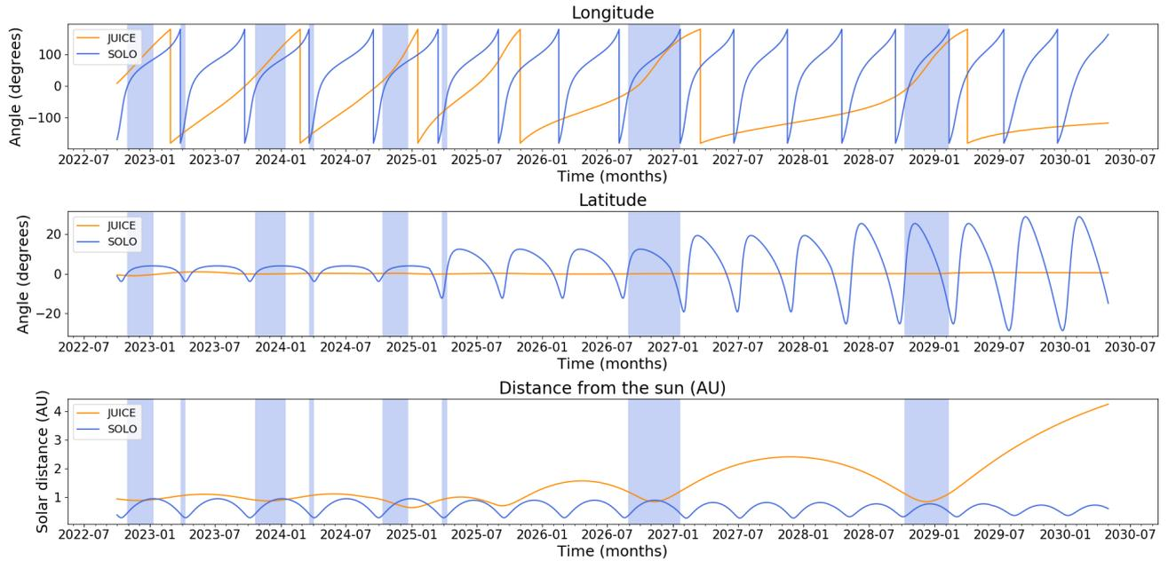
Figure 3.5: Longitudinal alignment between JUICE and Solar Orbiter within 45 degrees and at a maximal spacecraft separation of 0.83 AU. Areas of overlap have been coloured light blue. Note that these marked periods offer a window of opportunity to study the solar winds latitudinal variation.
