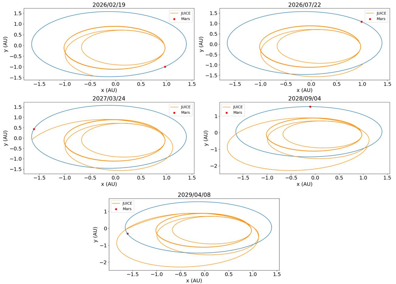
Figure 3.9: Crossing points of JUICE with the orbit of Mars at the respective dates. After launch, the spacecraft crosses through the orbit of Mars 5 times. Two times while moving inwards and three times while oriented outwards, with respect to the Martian orbit.
