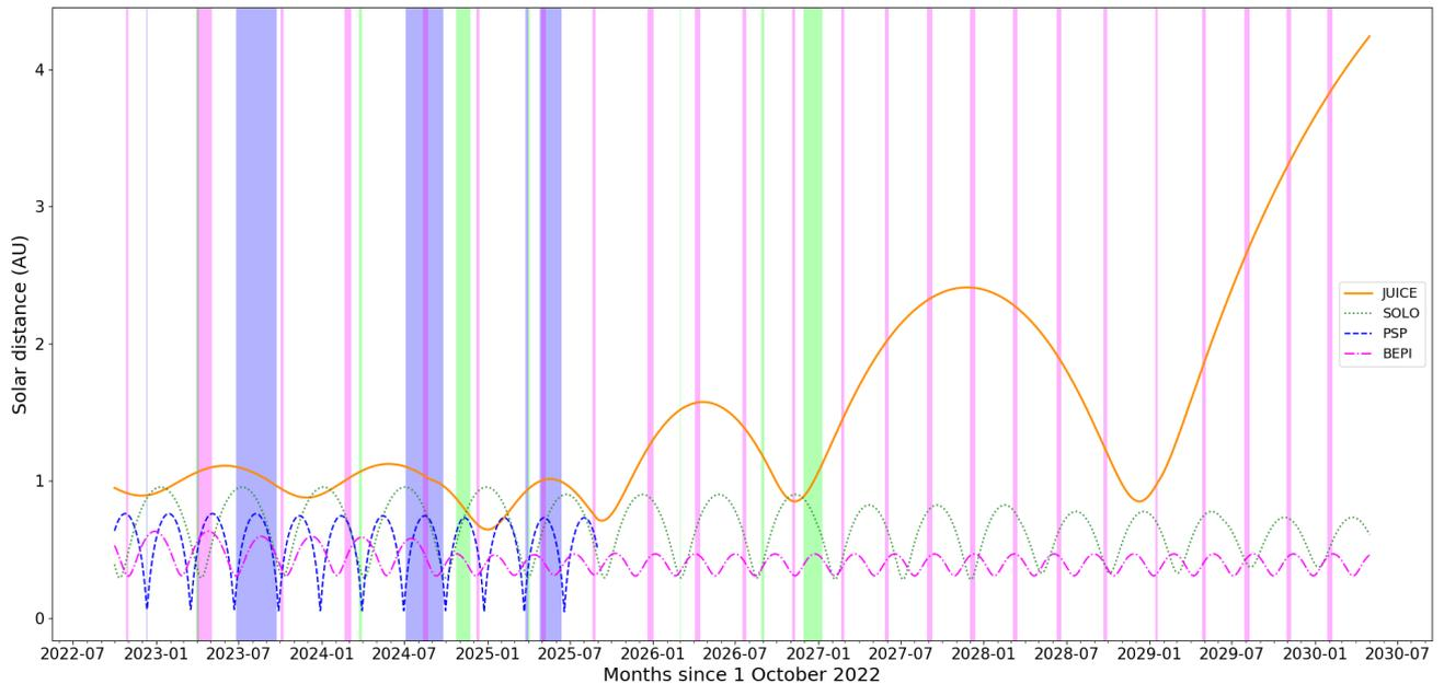
Figure 3.4: Radial alignment between JUICE and the other spacecraft within an angular separation of 15 degrees. The periods of alignment are marked in the colour of the respective spacecraft that is in conjunction with JUICE at that moment.
