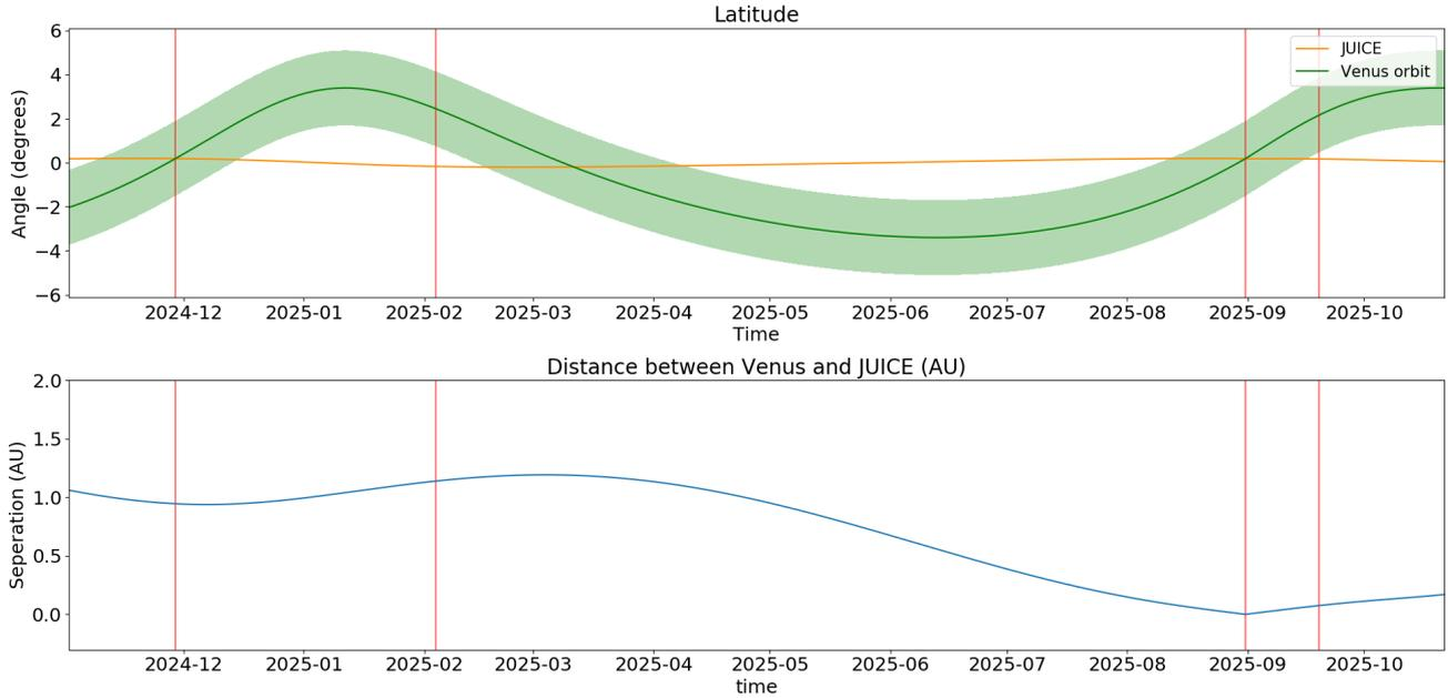
Figure 3.8: **Upper figure:** The latitude of JUICE and the Venus dust halo. The latitudes for the orbit of Venus are taken at the same longitudes as JUICE. The green region around the line of the Venus orbit indicates the extent of the dust halo. The red lines mark the moments at which JUICE crosses the orbit of Venus. **Bottom figure:** The distance between JUICE and Venus. The second-last crossing marks JUICE's Venus flyby.
