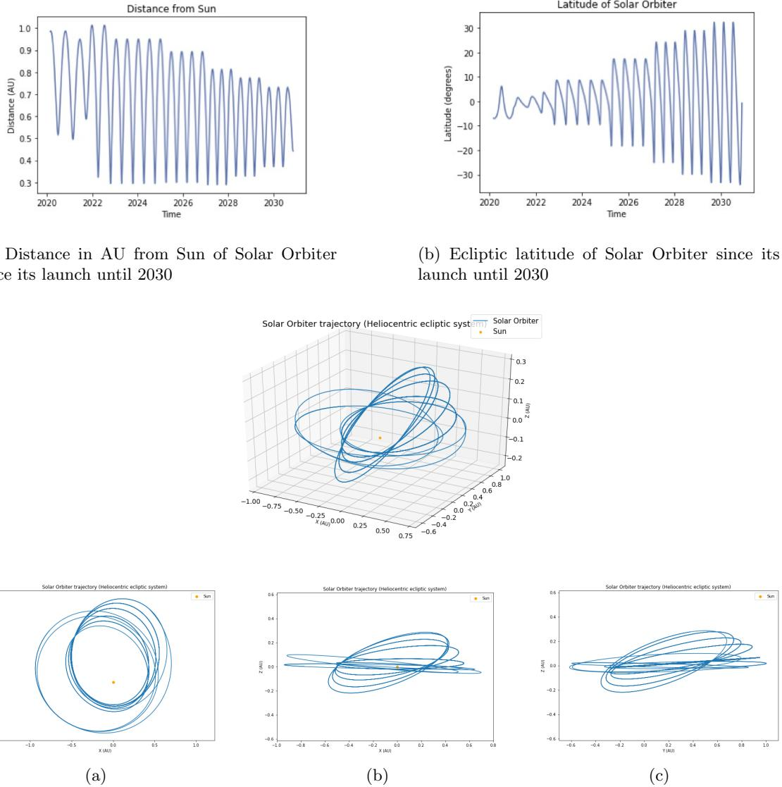
Figure 8: Solar Orbiter's trajectory in the heliocentric ecliptic coordinate system, since its launch until 2030. View in 3D (upper graphic) and 2D for every set of two coordinates: (a): Y vs X, (b): Z vs X and (c): Z vs Y. The Sun is represented by the orange dot. *Images source: Python program by the author.*
