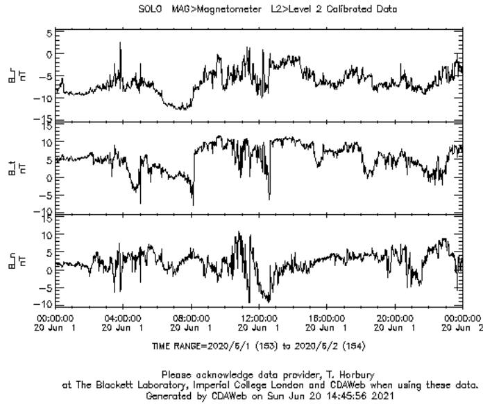
Figure 16: Magnetic field coordinates measured by Solar Orbiter in 2020 JUN 01.
