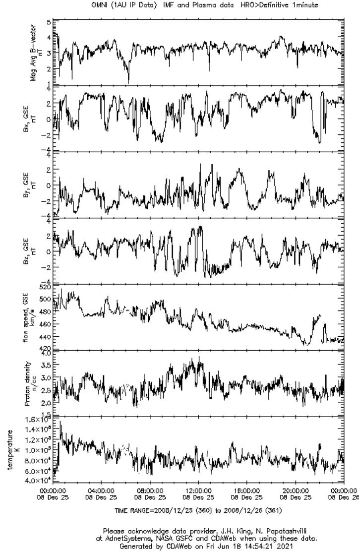
Figure 19: Magnetic field magnitude, magnetic field coordinates, solar wind speed, proton density and temperature from OMNI for date 2008 DEC 25.
