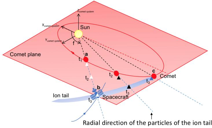
Figure 12: Drawing of the disposition of the spacecraft and the comet, showing the ion tail, at an encounter. Note that, for reasons of figure clarity, the comet has been drawn as moving at almost as high speed as the solar wind. A more realistic relation between the speeds will give an almost radial tail, but the principle is the same. *Image source: Drawn by the author.*
