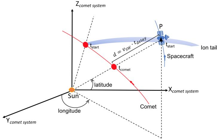
Figure 13: Drawing of the position of a point of the ion tail at a specific time. *Image source: Drawn by the author.*
