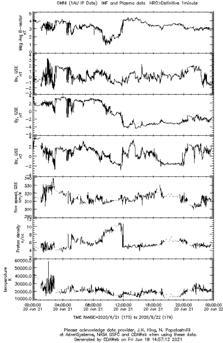
Figure 21: Magnetic field magnitude, magnetic field coordinates, solar wind speed, proton density and temperature from OMNI for date 2020 JUN 21.
