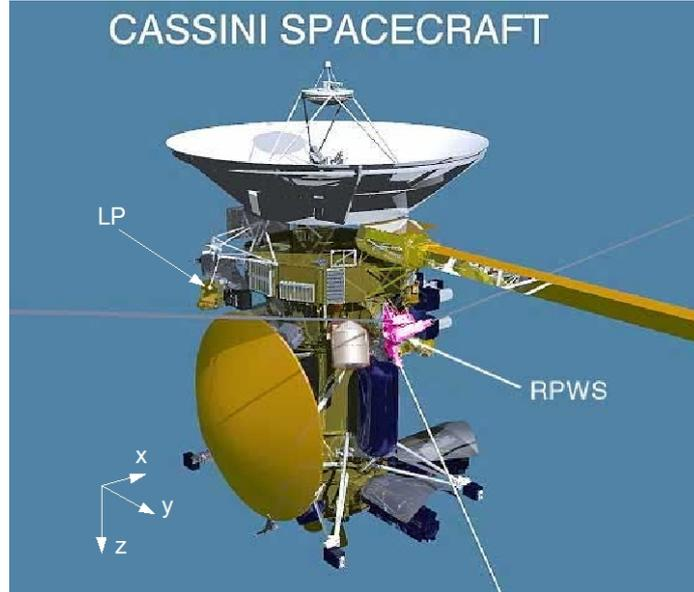
**Figure 3:** The Cassini-Huygens spacecraft. The Langmuir probe (LP) is mounted almost in negative  $X_{s/c}$ -direction. The gold-coloured part below the LP is the Huygens probe. Source: <http://saturn.jpl.nasa.gov/spacecraft/cassiniorbiterinstruments/nstrumentscassinirpws/images/rpws1.jpg>
