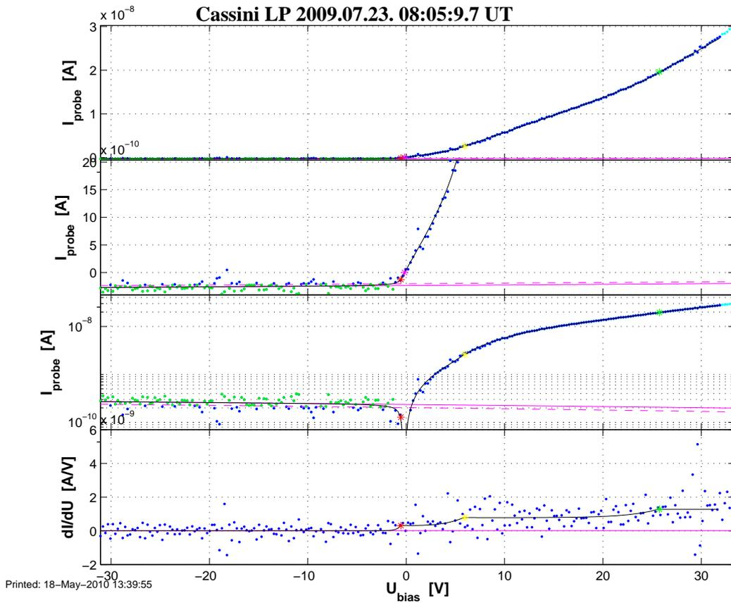
**Figure 4:** Typical Langmuir probe sweep, the left part ( $U_{bias} < 0$ ) is dominated by ions, whereas on the right part ( $U_{bias} > 0$ ) the current is mainly caused by electrons. The upper three panels show the current to the probe dependent on the bias voltage. The lower shows the derivative  $\frac{dI}{dU}$ . The floating potential  $U_{float}$  is marked with a red star \*.
