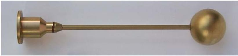
**Figure 23:** One of the two LAP probes, to scale (by courtesy of IRF Uppsala).
