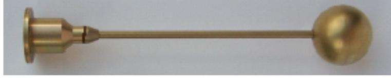
Figure 3.1: One of the two Langmuir probes on Rosetta
