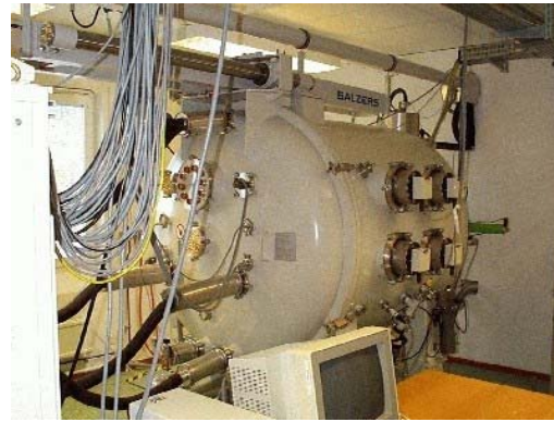
Vacuum chamber for space environment Thermal, outgassing tests, IRF Kiruna
