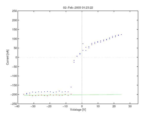
Fig. 1. A probe bias voltage sweep from Probe 2 of the EFW instrument on Cluster spacecraft 3, acquired on February 2, 2003, at 01:23:22 UT.
