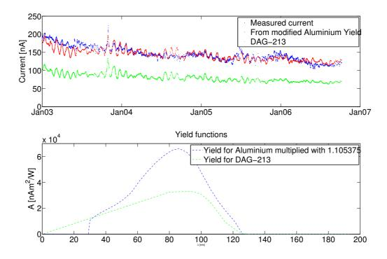
Fig. 2. Upper panel: The photoemission saturation current as measured by Cluster/EFW probe number 2 on Cluster spacecraft 3 (blue) and calculated from TIMED/SEE UV data using a yield function for aluminium (red) and DAG-213 (green). Lower panel: The yield functions used. The yield function for DAG-213 has been linearly extrapolated by us below 80 nm.
