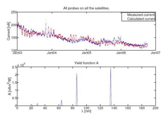
Fig. 3. Upper panel: The photoemission saturation current as measured by Cluster/EFW probe number 2 on Cluster spacecraft 3 (blue) and calculated from TIMED/SEE UV data using a yield function determined from all probes on all Cluster satellites, shown in the lower plot.
