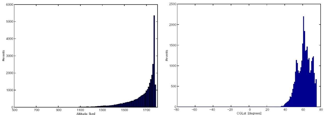
Fig. 2. The Freja coverage coverage of altitudes (left) and corrected geomagnetic latitudes (right) during its almost three years of operational lifetime. The histograms were made by dividing each ground station pass (15 – 30 minutes) into four intervals, using the positions at their centres.
